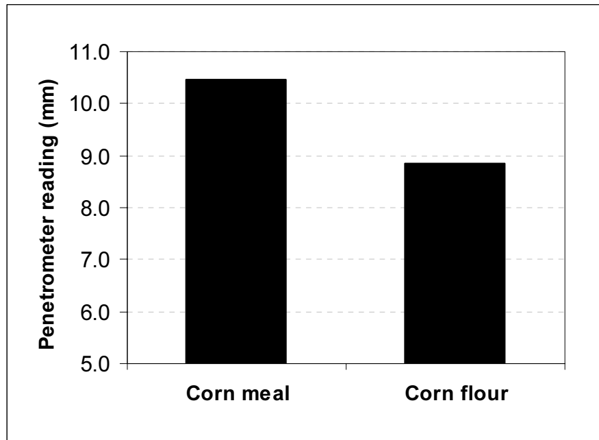
Fig. A-3. Texture quality (softness) of fresh corn porridges based on penetrometer readings.
