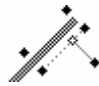
Fig 25 – The distances from each point to the intersection point (hollow) are shown as dashed lines, which the distance from the point of interest is a solid line
