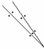
Fig 30 – An example of a case requiring mid-point examination due to misaligned bracketing points in close proximity
