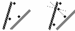
Fig 28 – Different line slopes result in a point which is not perpendicular to the intersection
