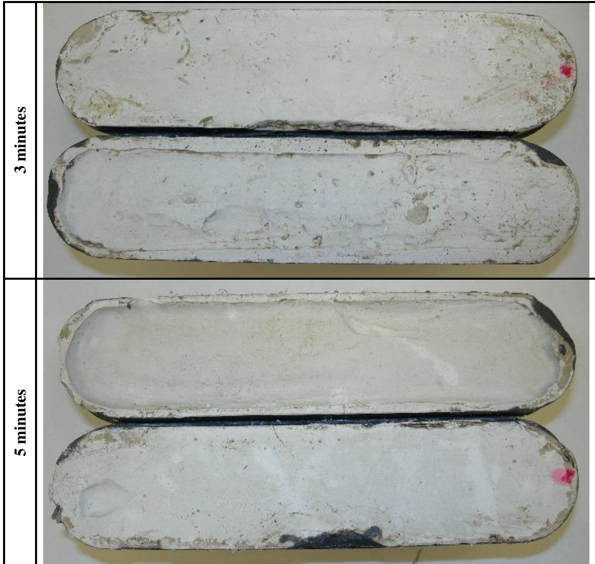
Fig. C-6—Exp. 7: Straight acid and chalk I, 100 °F, 0.005 ft/min.
