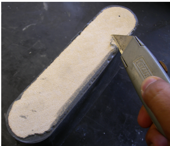
Fig. A-3. Cleaning the rock surface.
