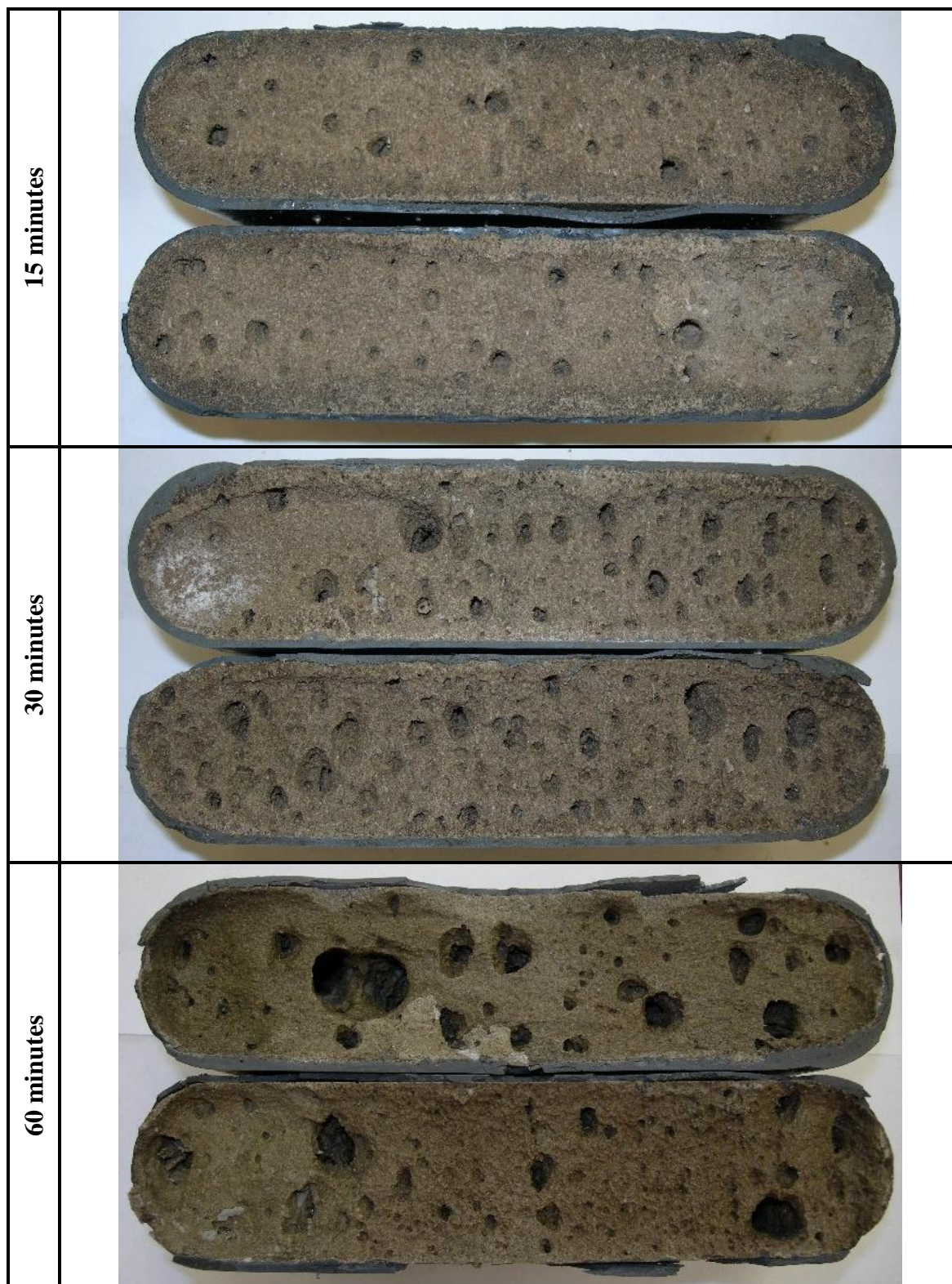
Fig. C-2—Exp 2: Emulsified acid and limestone, 275 °F, 0.005 ft/min.
