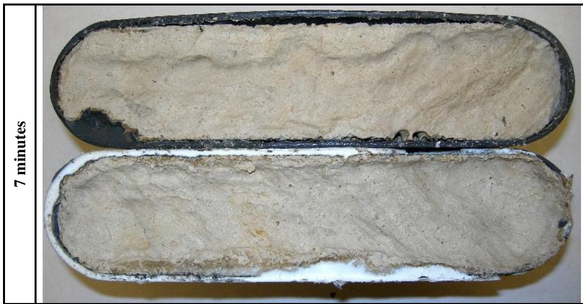
Fig. C-7—Exp. 8: Straight acid and chalk II, 100 °F, 0.005 ft/min.
