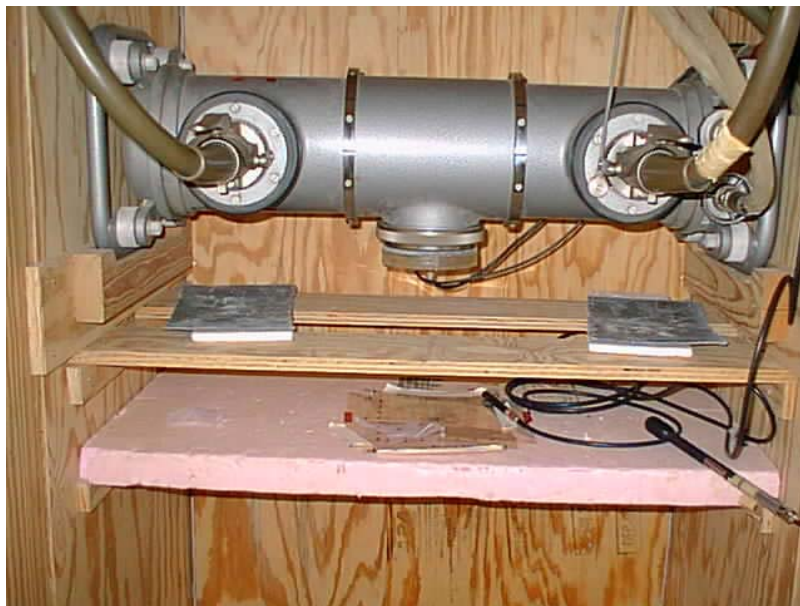
Figure V-7. X-ray machine (Norelco MG300) of the Nuclear Science Center
