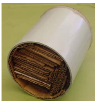
Fig. 2. PVC pipe and corrugated cardboard bait station used to collect Reticulitermes spp. termites on a weekly basis.
