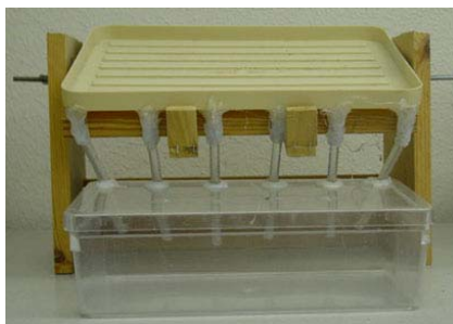
Fig. 3. Stage-tube-box system is used to remove the dirt and debris from the termites. Slowly the termites trickle down the sloped stage and through the tubes into the plastic box for collection.
