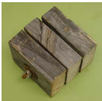
Fig. 1. Wooden sandwich bait station, used specifically to capture foraging Coptotermes formosanus termites in Baytown and Beaumont, Texas.
