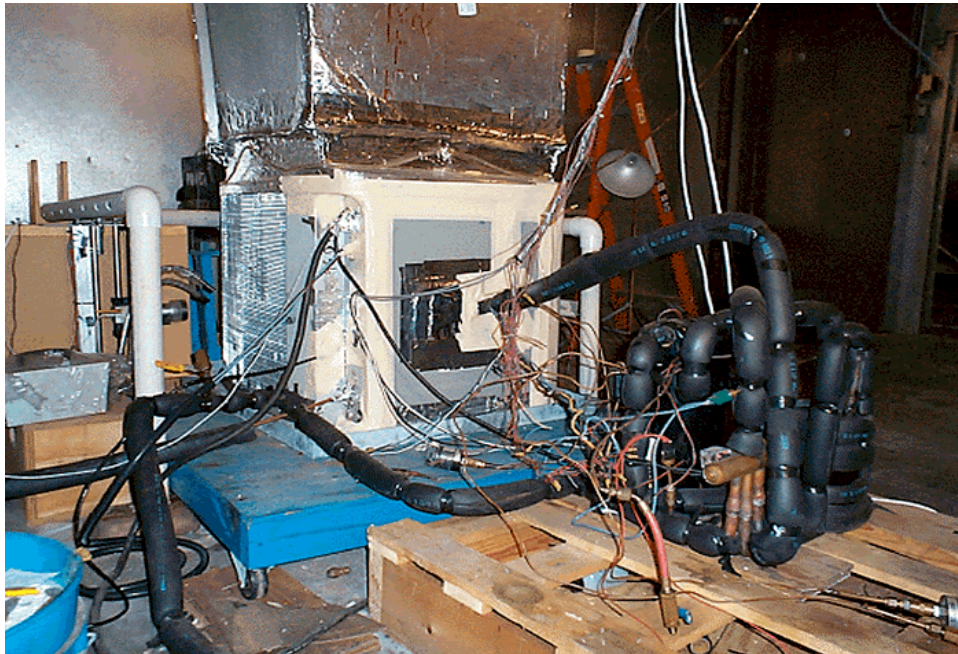
Figure 3.15 The outdoor coil with the compressor, accumulator, and reversing valve moved out
