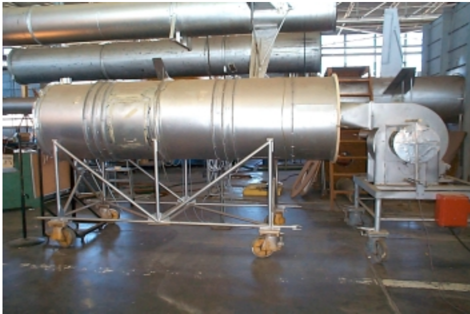
Figure 3.33 Multi-nozzle inlet fan test chamber at Energy Systems Laboratory
