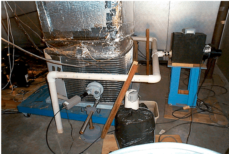
Figure 3.20 Air-sampling pipes and mixing box setup around the outdoor coil
