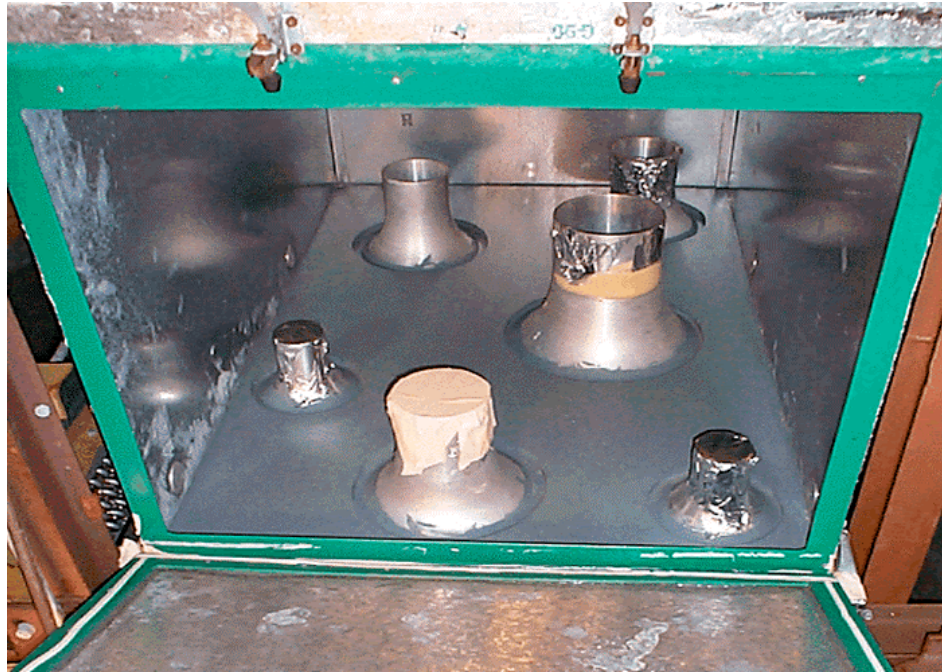
Figure 3.22 The nozzle plate of the outdoor airflow test chamber
