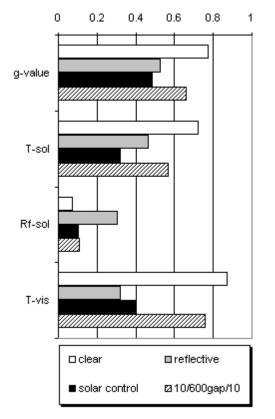
Figure 5. Glazing properties of glazing types used
