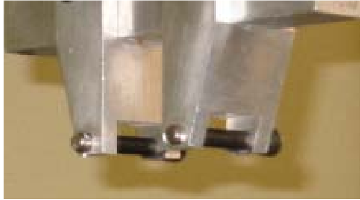
Figure 6. Upper fixture consisting of roller load application for flexure experiments
