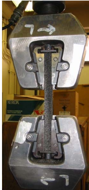
Figure 18. Direct grip fixture for tension experiments
