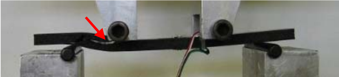
Figure 14. Damage initiation crack in sandwich specimens
