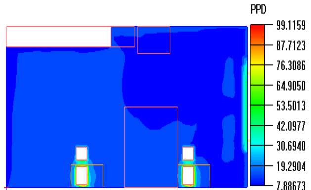
Fig. 25 PPD distribution in 1.1m above the floor at inlet area 0.30m 2
