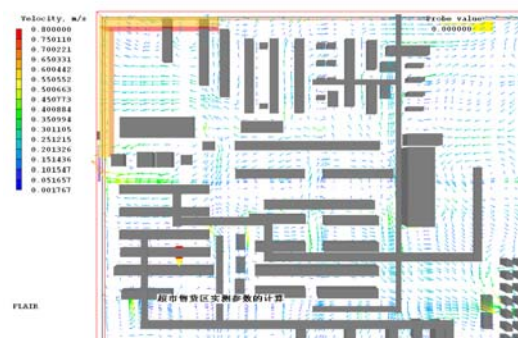
Fig.3 Air velocity distribution at 0.4m height
