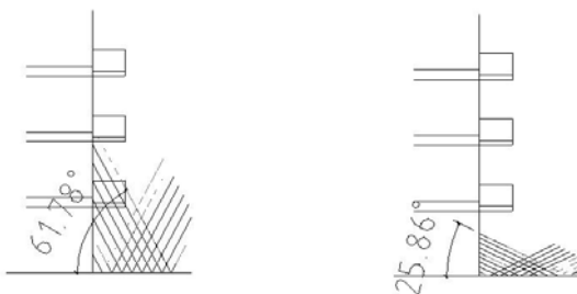
Fig.4.Floor between buildings Fig.5.Floor between buildings glint to heat from to sun buildings glint to heat radiation in northern from sun radiation latitudes 34^\circ in the summer solstice day at 14:00 34^\circ in the winter solstice day at 14:00
