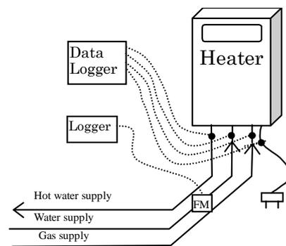
**Fig.7. Measurement setups**
