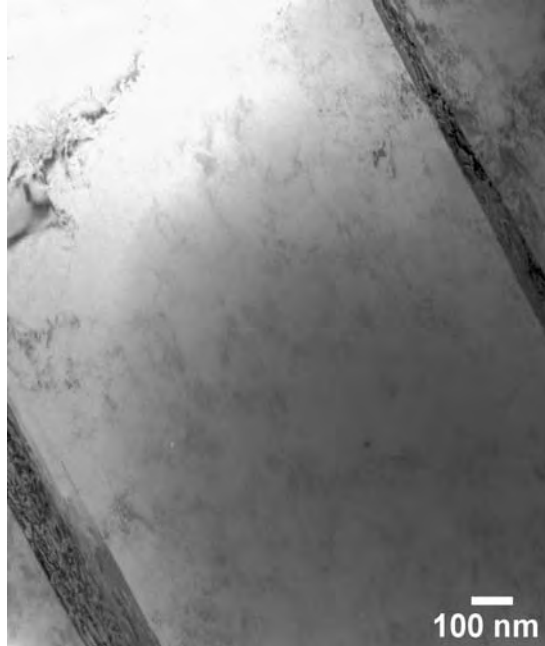
Fig. 5.1.4. TEM micrograph of SS 316L as-received material demonstrating dislocation free regions with annealing twins.
