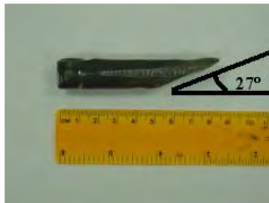
Fig. 3.1.2. Single pass Ti-6Al-4V processed non-isothermally in a stainless steel can at 800°C.
