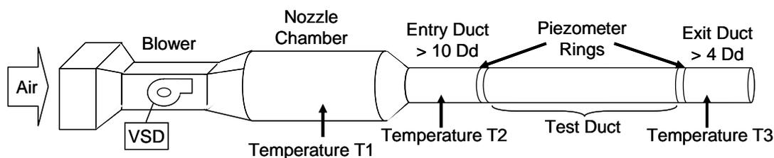
Fig.1 Test Setup
