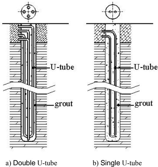
**Fig.1 Schematic diagram of boreholes in the vertical GHE exchanger**
