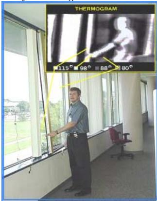
The prior Photo and Thermogram is of a **Interior Storm Window Daylighting Retrofit** at a U.S. Naval Station, you will note some of the Load Data Recording devices are still attached to the building envelope. The following Figures, 4 & 5 show a synopsis of some of the results from this field survey. We have obviously made a positive impact on light levels without adding any additional discomfort factors.
