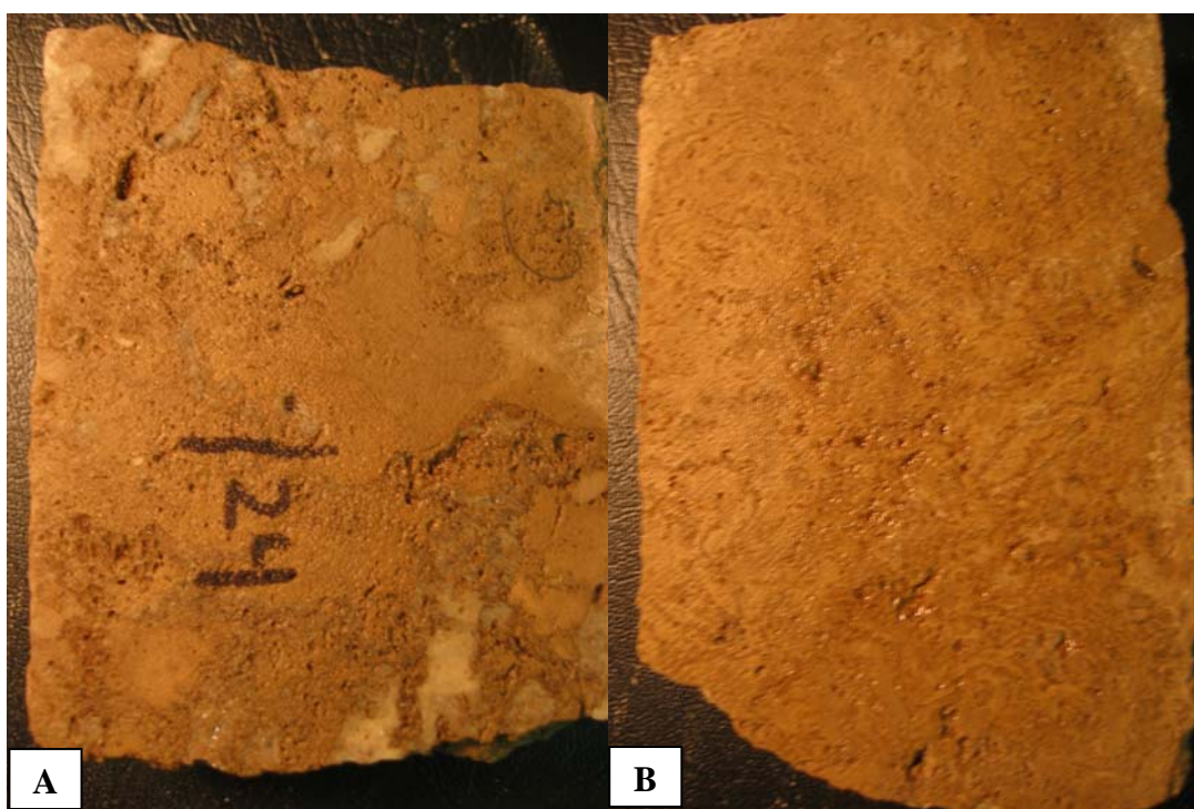
Figure A-1. A) Core photo taken from Reeves # 1 @ 8024' representing the Microbial Boundstone Facies as well as abundant replacement. B) Core photo taken from Reeves # 1 @ 8027.5' representing microbial boundstone facies exhibiting a thombolitic texture.
