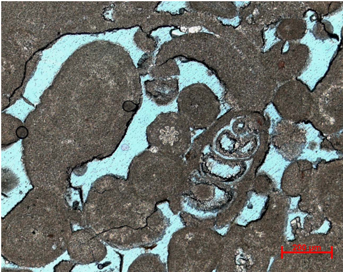
Figure B-1. Thin section photo from Alexander #1 @ 8056.0'. Extensive micritization and leaching visible.
