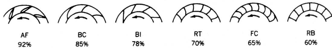
Figure 13: Common centrifugal fan blade shapes.
