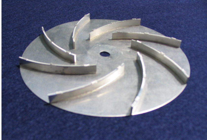
Figure 9: Turbo blowers with backward curved blades (shroud removed).
