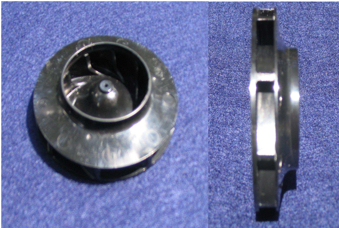
Figure 10: Hand-held vacuum system centrifugal blower (a) Top-view (b) Side-view showing the blades.
