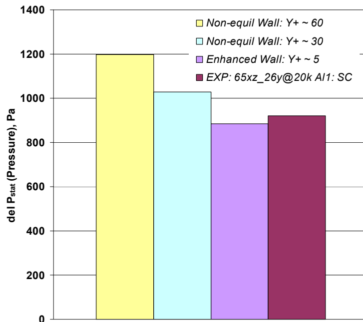
Figure 37: FLUENT static pressure rise value for 65xz_26y blower for different wall treatments and comparison with Al-1: SC experimental data.
