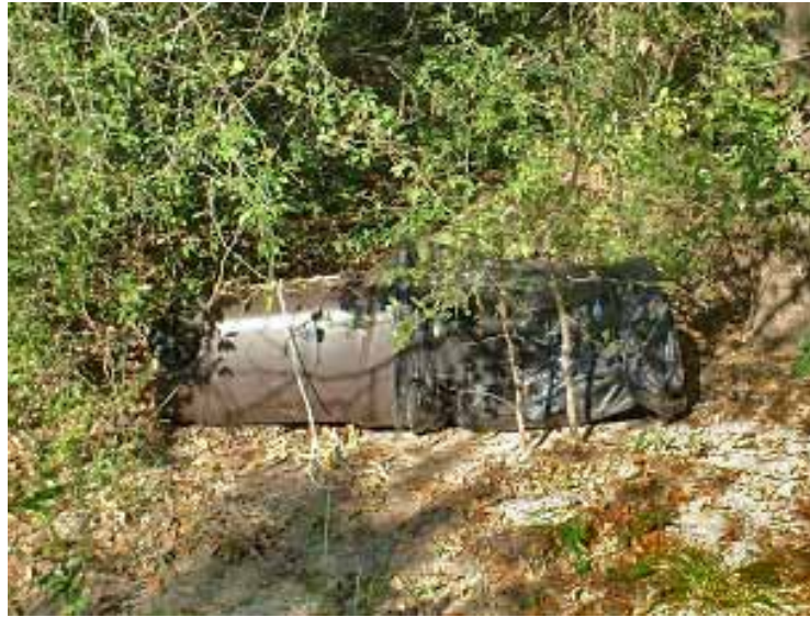
Figure1. Picture depicting an artificial adult mosquito resting site trap out of which adults can be aspirated during the day. This trap consists of a brown or red trash can, wire mesh covered lid, and black trash bag extended out from the opening that is held up by a tomato cage.
