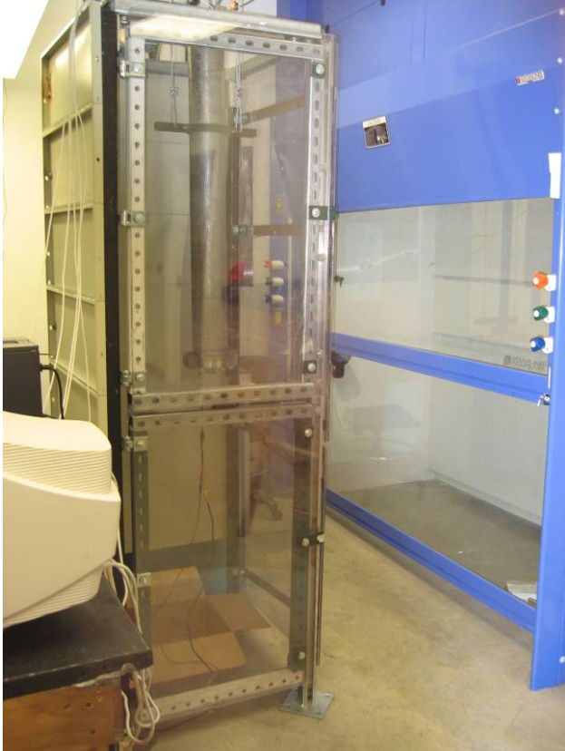
Fig. 4.5. Reaction vessel enclosure front view.
