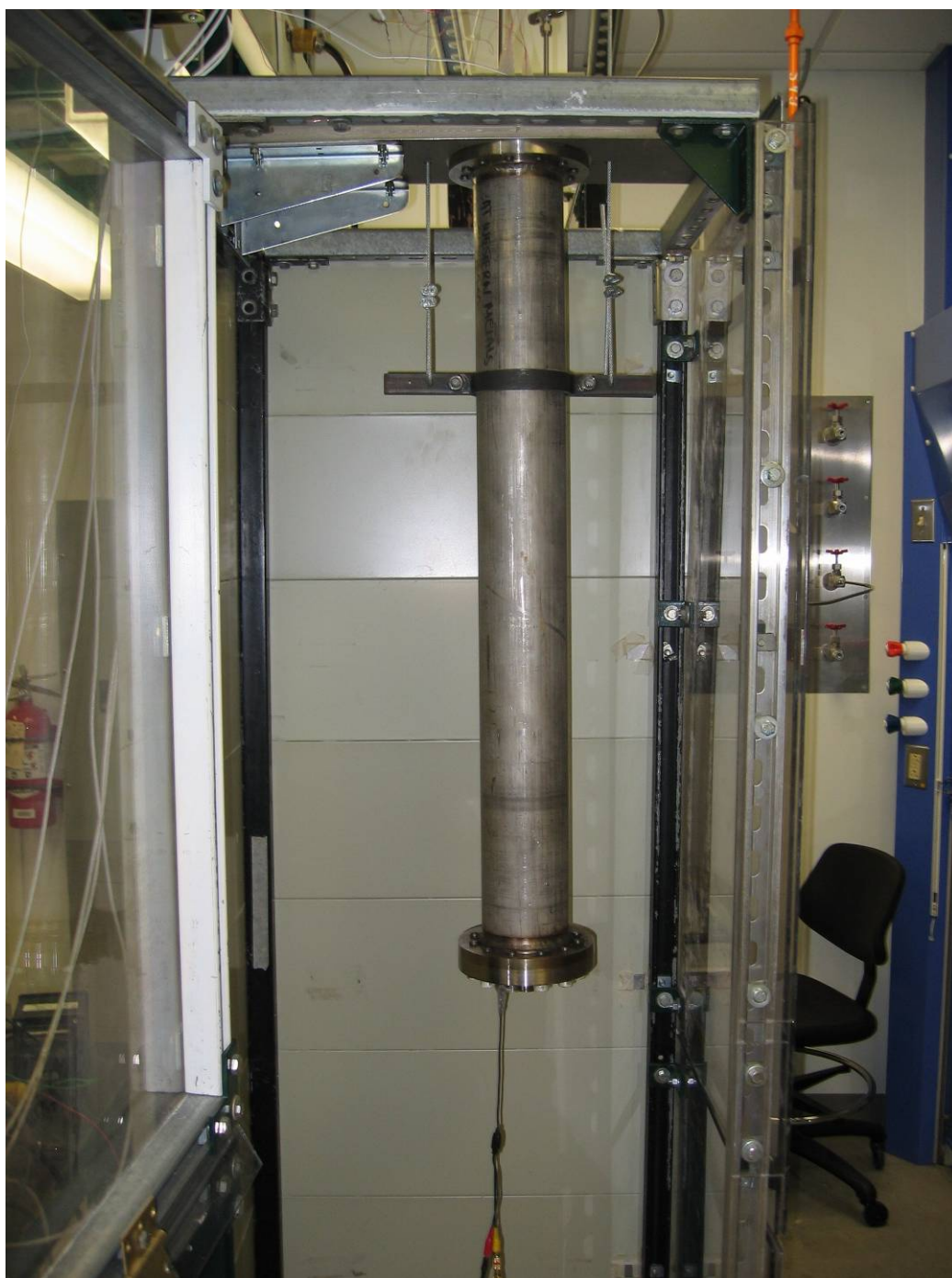
Fig. 4.2. Reaction vessel mounted in the safety enclosure.
