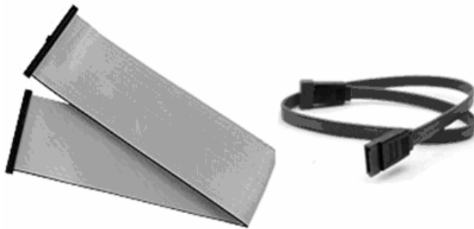
Fig. 1.1. Comparison of a parallel ATA cable and a serial ATA cable
