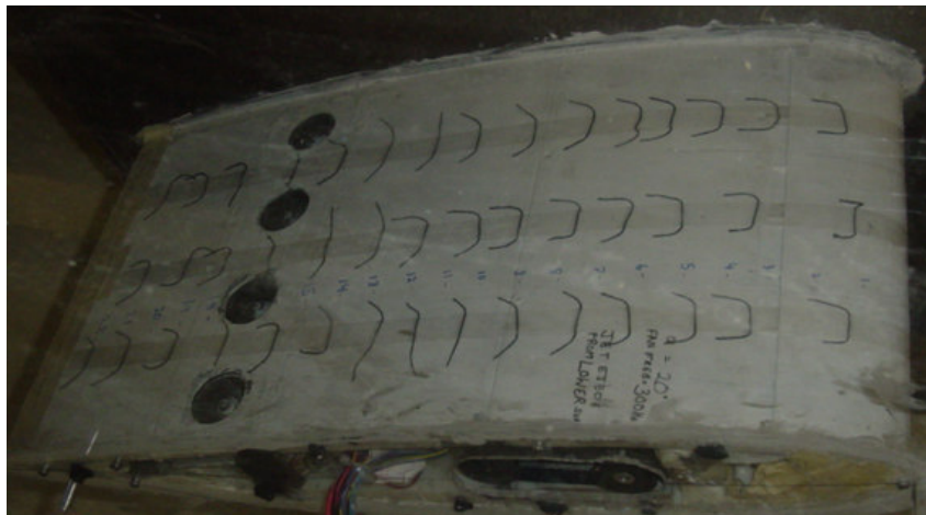
Figure 42: Tufts flow visualization of test wing. Trailing edge actuator control with jet ejecting from lower surface at 300 Hz.
