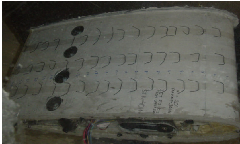
Figure 45: Tufts flow visualization of test wing. Trailing edge actuator control with jet ejecting from upper surface at 300 Hz and SJA control at 40 Hz.
