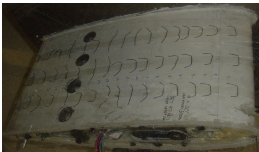
Figure 44: Tufts flow visualization of test wing. Trailing edge actuator control with jet ejecting from upper surface at 300 Hz.
