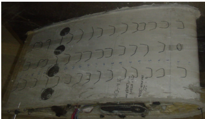
Figure 43: Tufts flow visualization of test wing. Trailing edge actuator control with jet ejecting from lower surface at 300 Hz and SJA control at 40 Hz.
