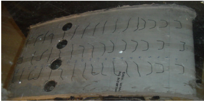
Figure 41: Tufts flow visualization of test wing. No control.
