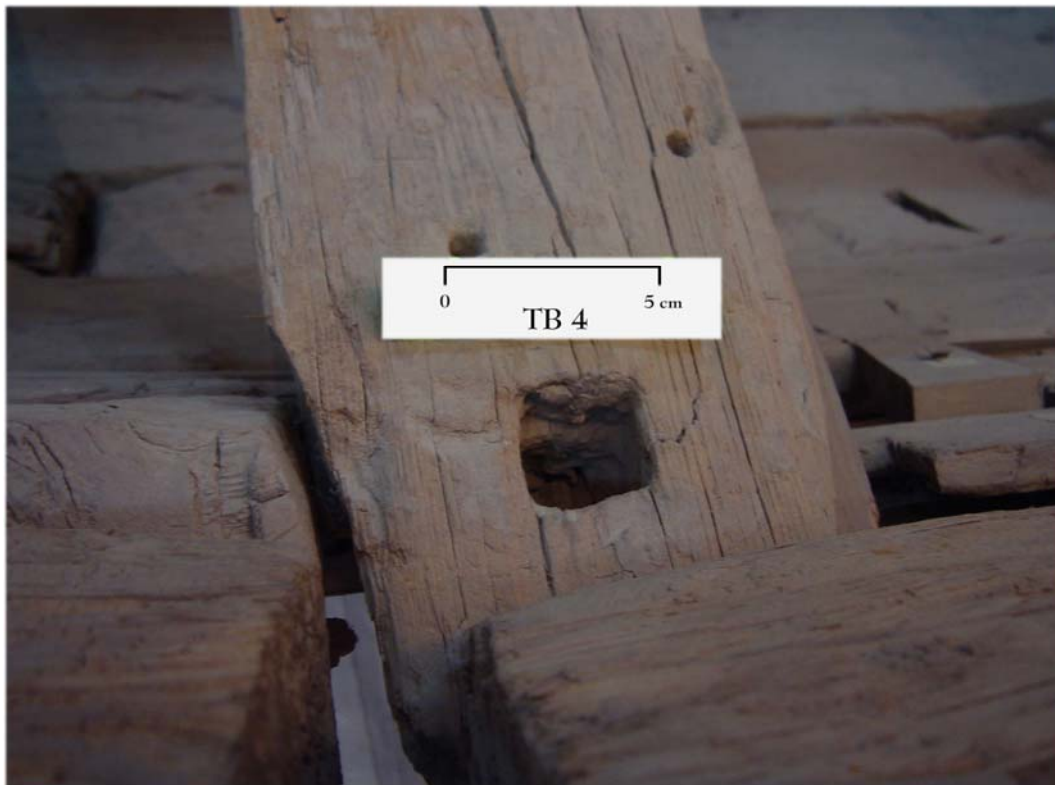
Figure 24. Starboard end on throughbeam 4 of the de Morgan boat showing narrowing (P. Creasman).
