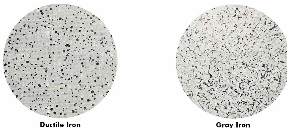
Fig. 3.11--Photomicrographs showing the graphite structure (DIPRA 2003).
