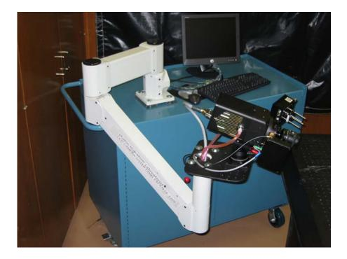
Figure 3.4 Photograph of the clinical ICCD camera system. Instrumentation resides in the interior of the cart, which is on casters for mobility around the nuclear imaging suite.
