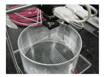
Figure 3.7 Photograph of cylindrical phantom with fiber optics inserted into the center for fluorescence depth measurements.
