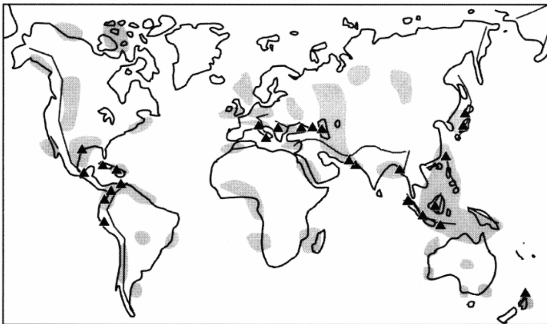
Figure 7 Tectonically influenced overpressure distribution on earth. Shaded regions represent where tectonically induced pore pressure is observed, lines represent where Cenozoic folding occurred, and triangles represent where mud volcanoes are observed. 6
