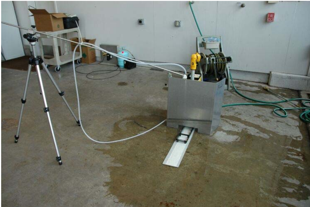
FIGURE 18 Tripod Setup with Retroreflectometer on Marking (Front View).
