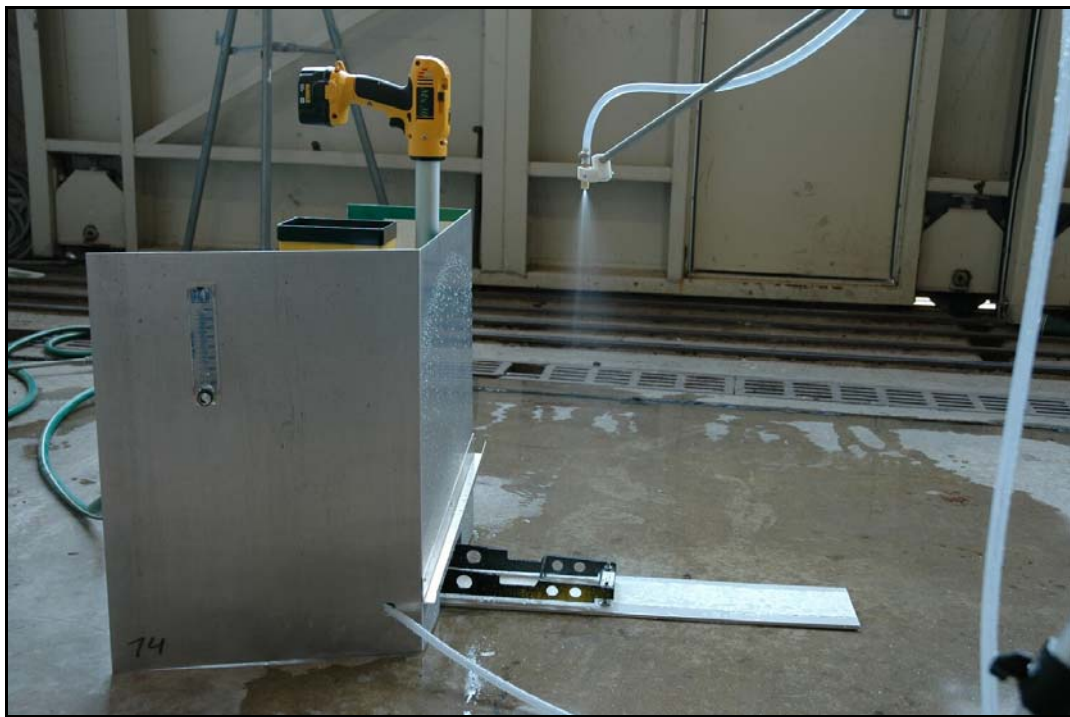
FIGURE 19 Retroreflectivity Data Collection Setup (Side View).
