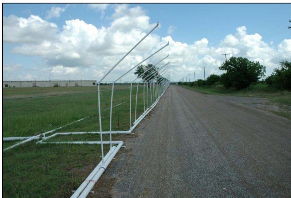
FIGURE 23 Midpoint of Rain Simulator (Dry).
