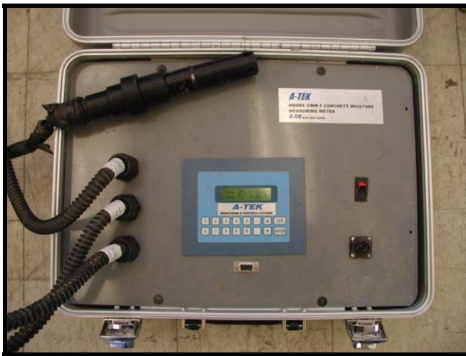
Figure 13 - Concrete Relative Humidity Moisture Meter and Embedding Sensor Probe
