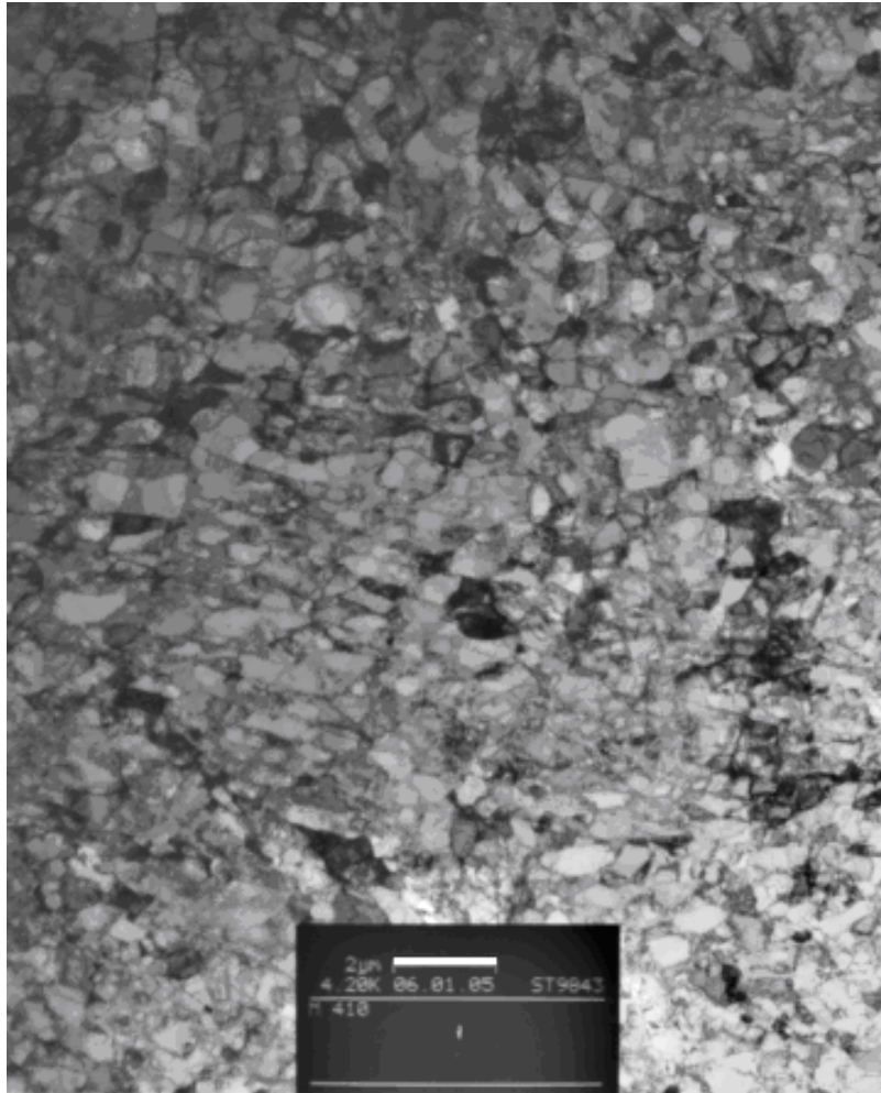
Figure 92: Low magnification TEM image of ECAE 4E IF steel (white bar = 2 \mu\text{m} )
