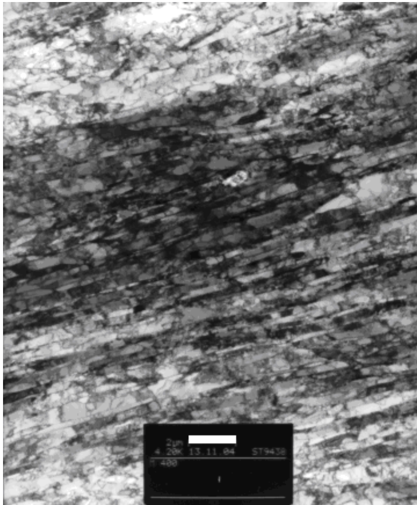
Figure 79: Low magnification TEM image of ECAE 2B IF steel (white bar = 2 μm)
