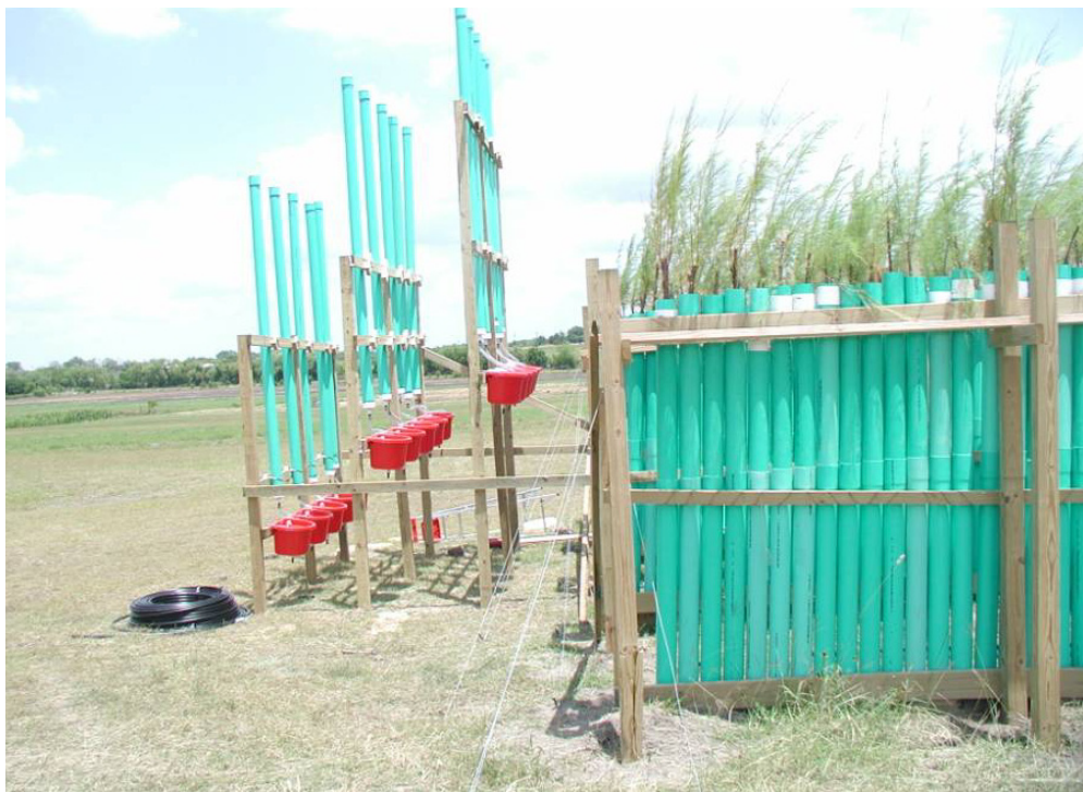
Figure 4. Photograph of lysimeter study, side view, showing different water levels.
