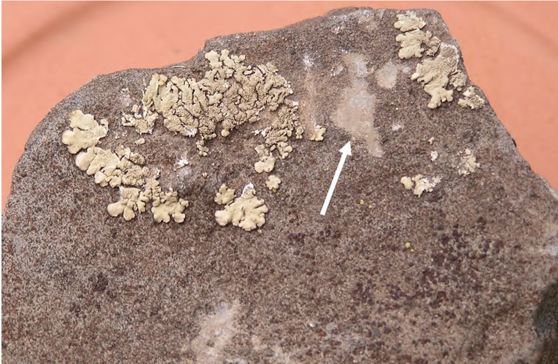
Figure 15. Example of “clean” appearance after lichen has been removed from the rock surface with tweezers.
