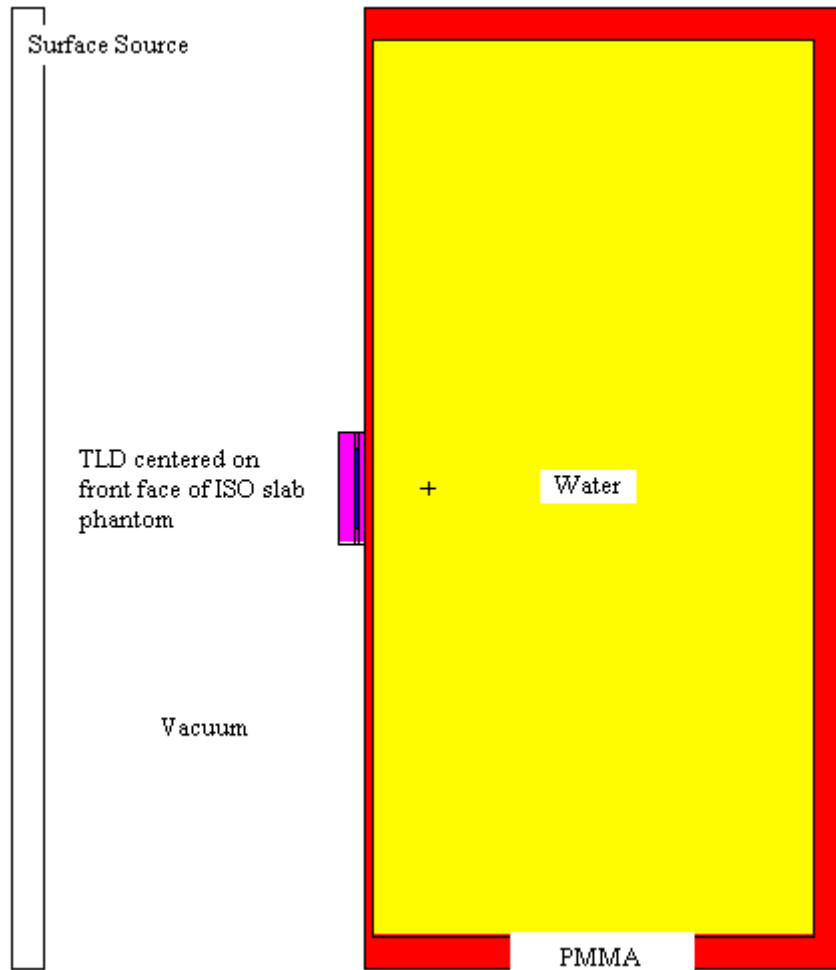
Fig. 10. Side view of MCNP geometry plot for problem 4.
