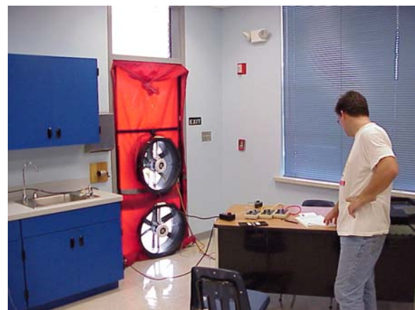
Figure 5 Blower door testing being completed on one of the classroom buildings.
