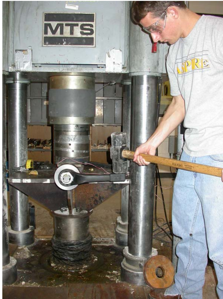
Figure 2.9 – Tightening with a slug wrench and sledgehammer
