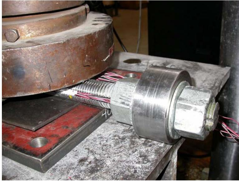
Figure 2.7 – Fully assembled bolt specimen
