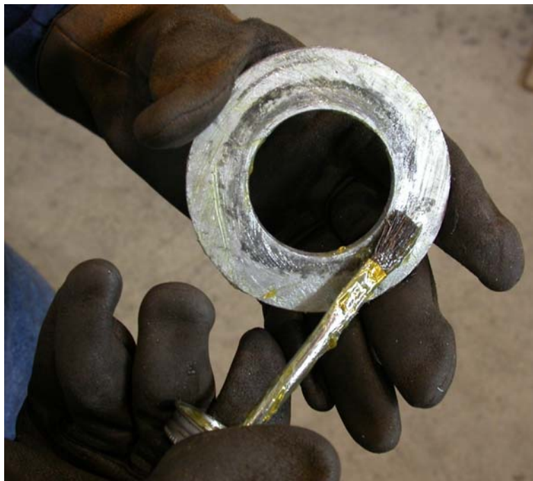
Figure 2.6 – Lubricating washer faces
