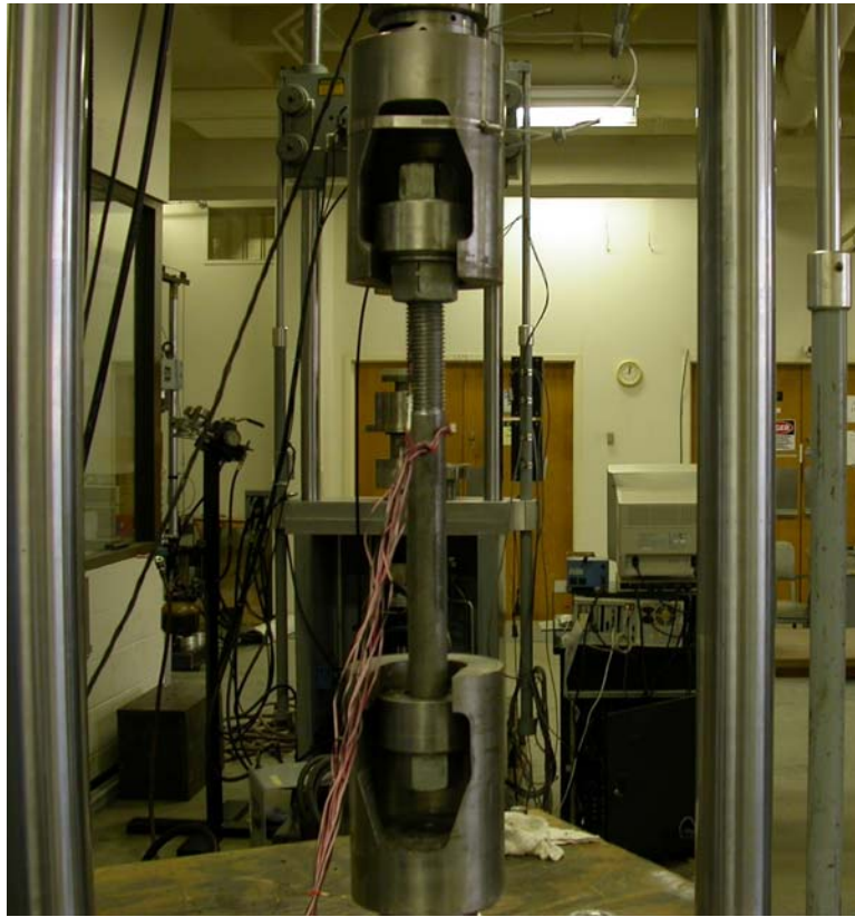
Figure 2.8 – Assembled bolt fatiguing in 100 kip MTS machine
