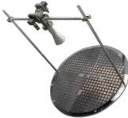
Fig. 4. A photo of the reflectarray with microstrip rings of variable rotations and a CP feed horn.
