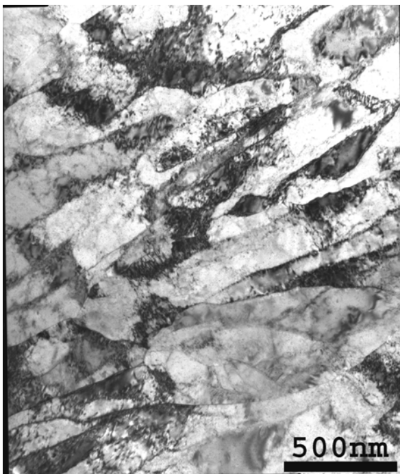
Fig. 76. TEM of CDA 101 Cu in as-worked condition along the flow plane of billet processed through route 2C in a 90° die.
