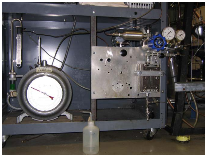
Fig. 3.6- Photograph of back pressure valve and wet test meter.
