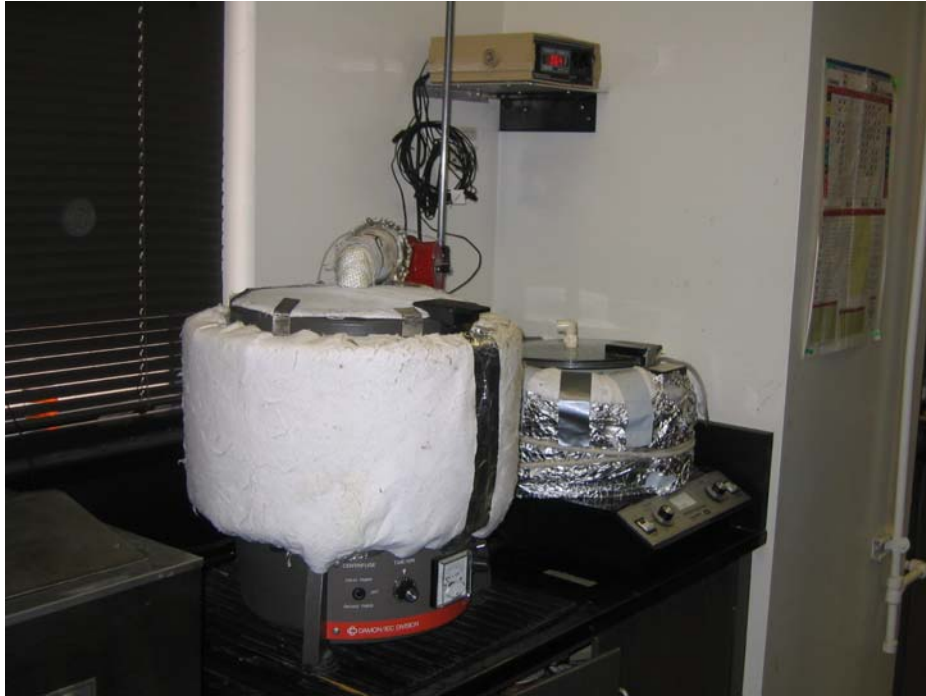
Fig. 3.11- Photograph of insulated centrifuge with heater gun to keep samples warm.
