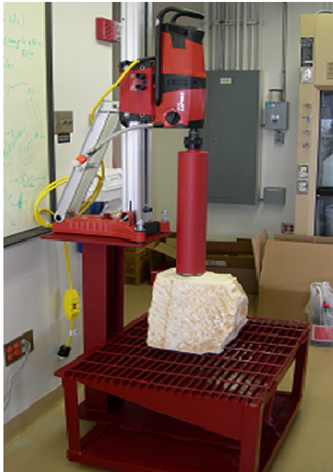
Figure 2. 17 Heavy duty HILTI DD200 core driller and core bits
