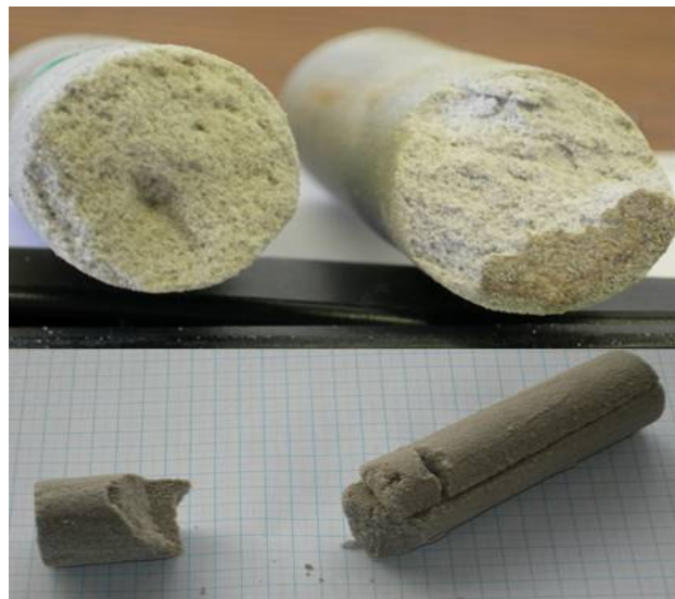
Figure 4.10 Inlet face of cores acidized with 9% HCl- 6% HF
