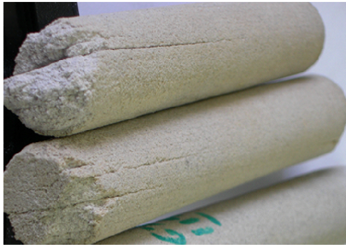
Figure 4.9 Dissolved minerals in bedding planes of the cores
