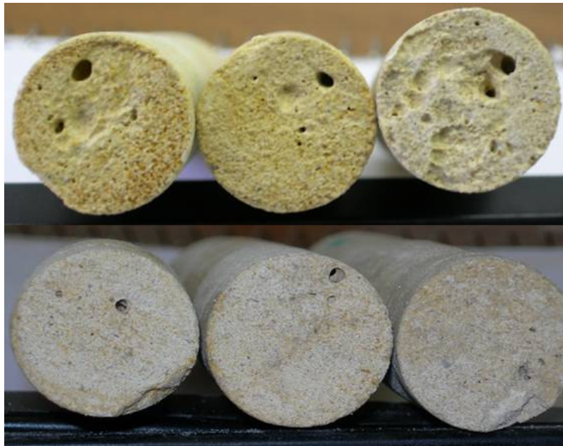
Figure 4.14 Wormholes at inlet and outlet face of carbonate cores
