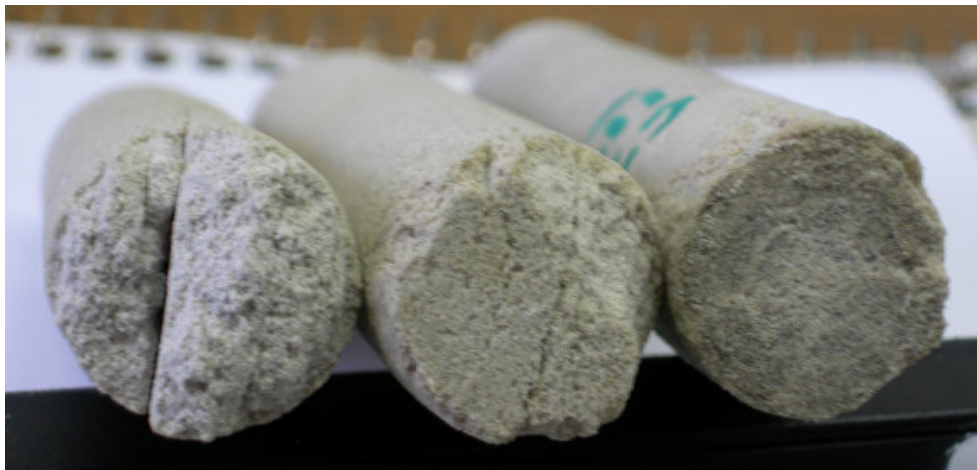
Figure 4.1 Inlet face of acidized Berea sandstone cores
