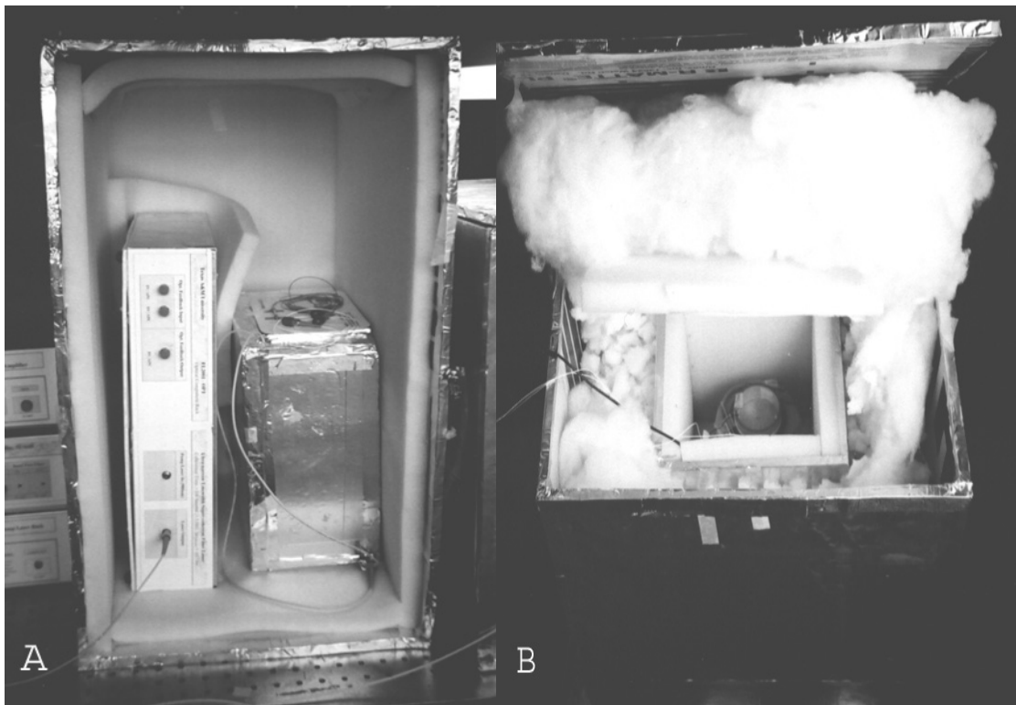
Figure 12. A) Laser and feedback path housing B) MZI housing
