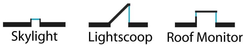
Fig. 3.3 Cross sections of toplighting systems
