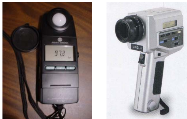
Fig. 3.21 An illuminance meter Konica Minolta T-10 and a luminance meter Minolta LS-100
