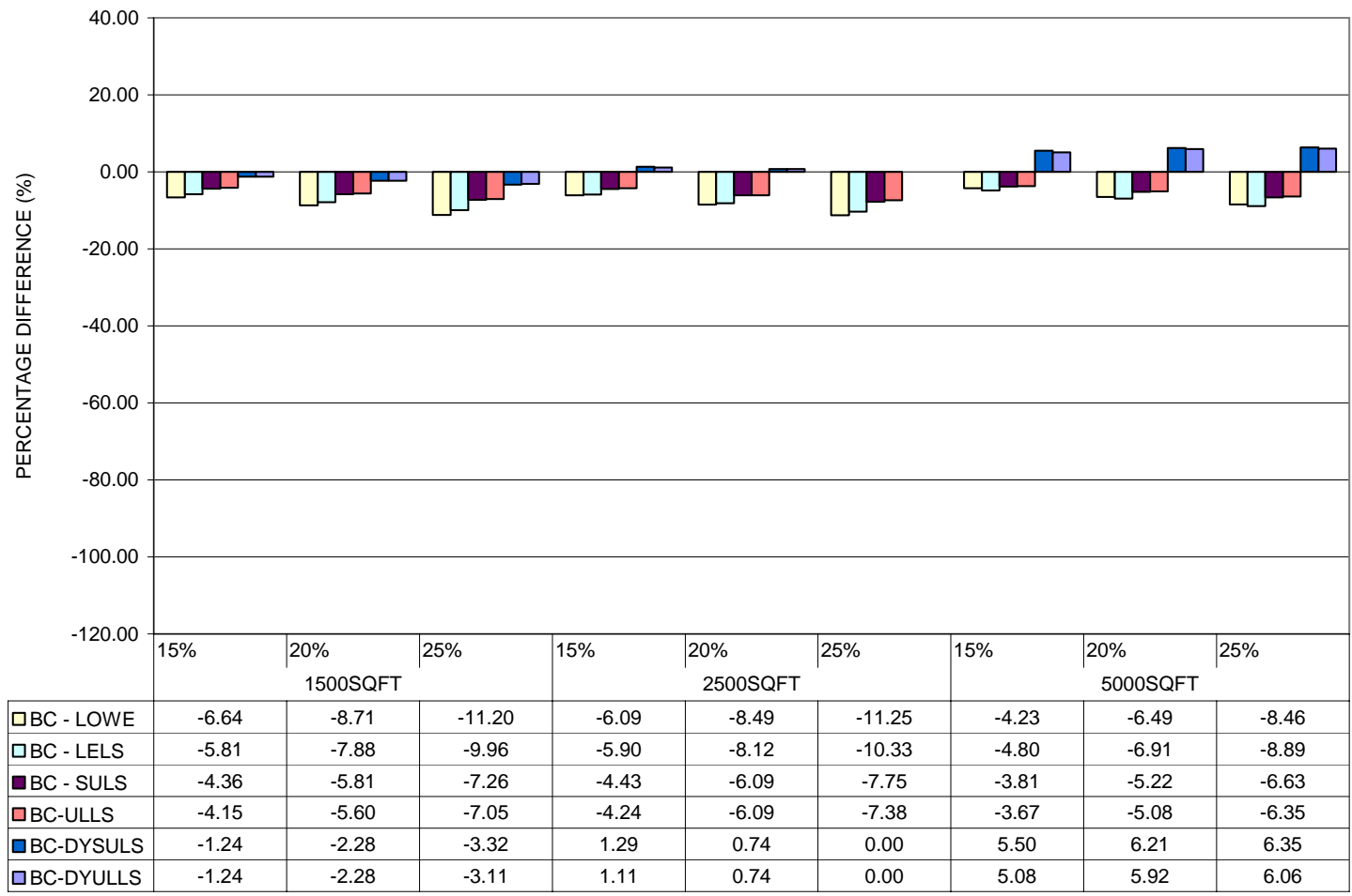
Figure B.17 Percentage difference between windowless base-case and high-performance options: Overall energy consumption
