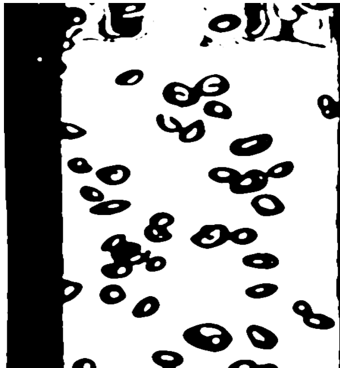
Fig.8. Typical Grade B Threshold Applied to a Shadow Image
