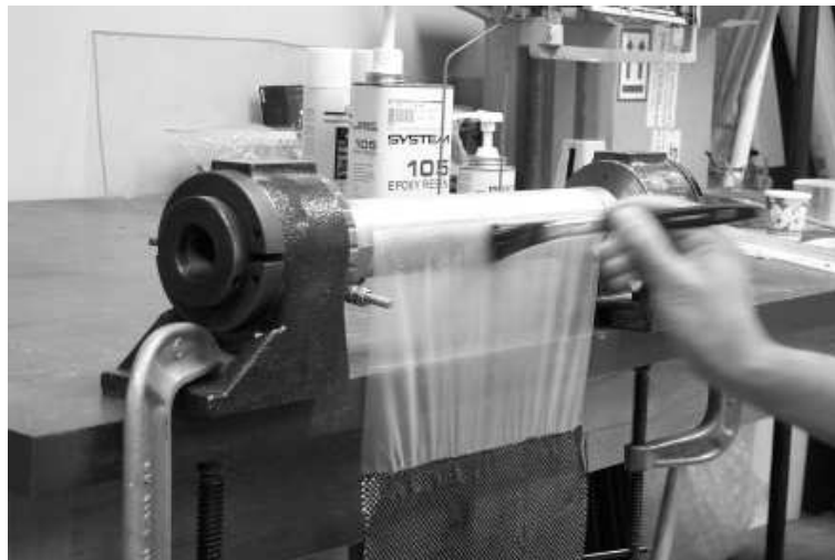
Fig. 33. Application of resin to polyethylene
