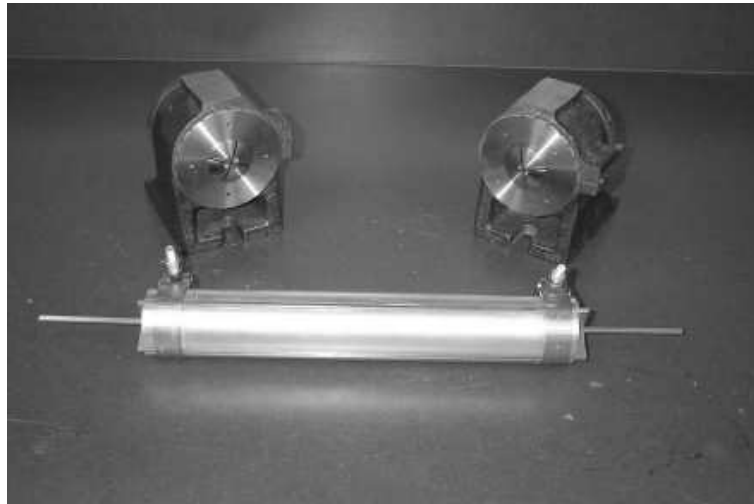
Fig. 27. Assembled mold and collet fixtures
