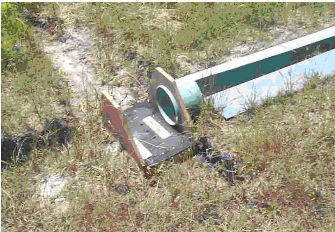
Figure 3.8. An installed collection pipe with the sampler at College Station
