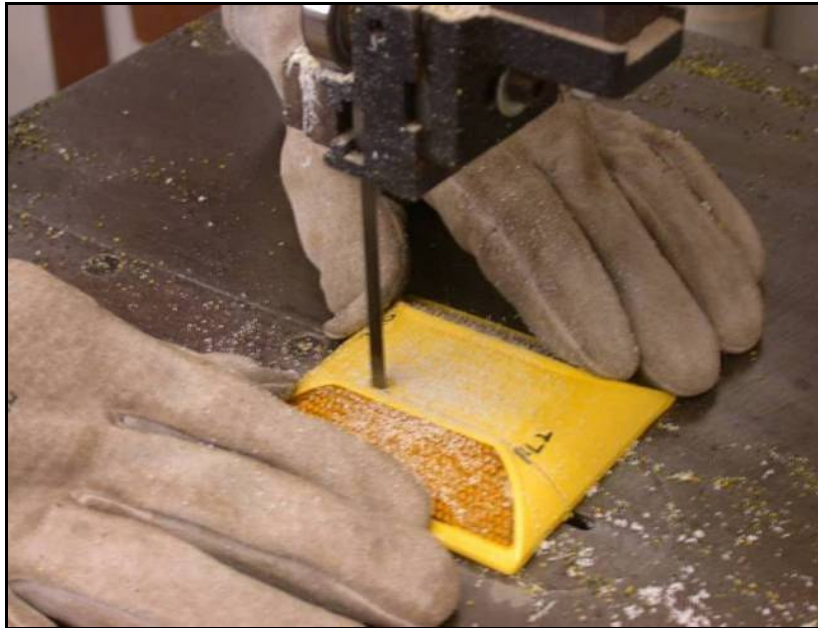
FIGURE 19 Marker body being cut.
