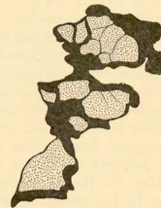
FIGURE 13.—Typical pyrite kernels in chalcocite. Schist ore, 1925 level of the No. 2 mine, Ray district.
