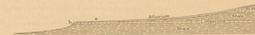
FIGURE 9.—Diagrammatic profile of stream bottom showing rapids or small cascade (b) below outcrop of thin resistant limestone bed and low gradient (a) above it.
