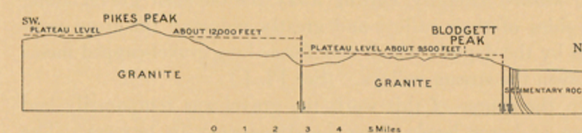
FIGURE 8.—Section through Pikes Peak showing dissected plateau representing the Tertiary peneplain displaced by the Ute Pass fault, the area about Pikes Peak having been relatively uplifted about 2,500 feet.
