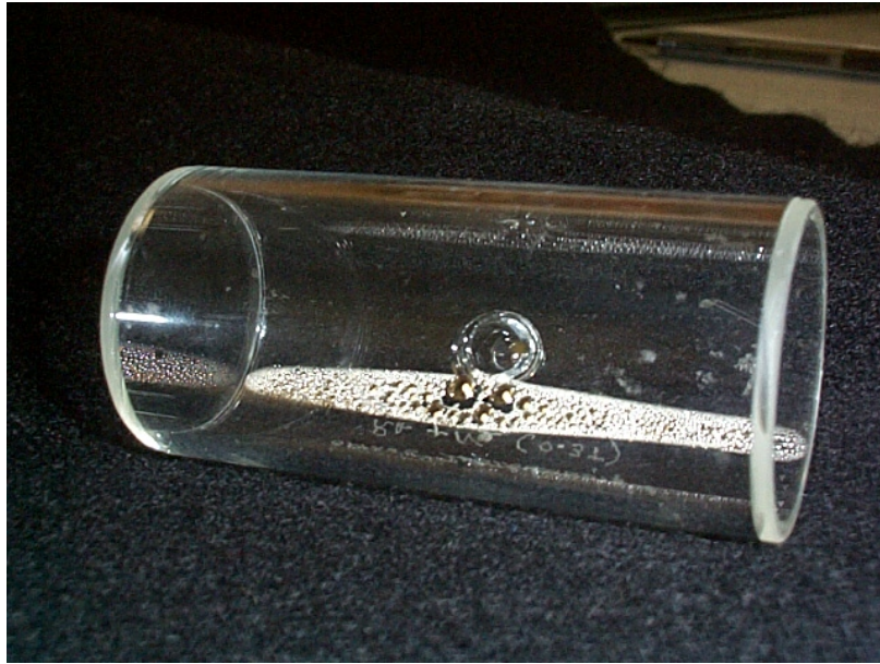
Fig. 69. Glass atomic cell with drops of liquid Rb.
