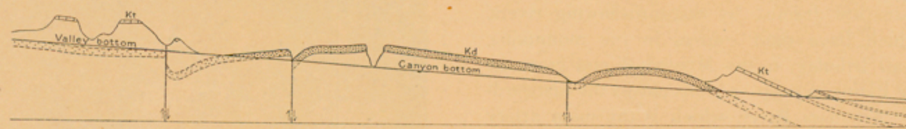
FIGURE 5.—Profile along Apishapa River in the Apishapa quadrangle. The river's canyon in the arched Dakota sandstone in the middle is flanked at both ends by open valleys in the softer overlying strata. Kd, Dakota sandstone; Kt, Timpas limestone. Horizontal scale: 1 inch = 4 miles. Vertical scale ten times the horizontal.
