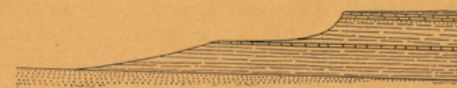
FIGURE 3.—Typical profile of the mesa escarpment capped by Timpas limestone, the medial bench capped by Greenhorn limestone, and the lower plain composed of Dakota sandstone.
